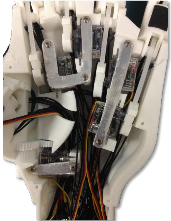
Figure 28: Installation of aluminum servo covers (left hand)
