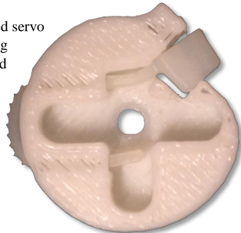
Figure 16: Zip-tie installed in servo spool
