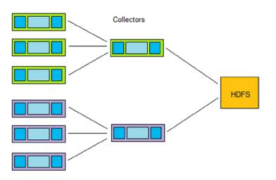
Figure 6-2. Hierarchical example of Flume architecture
