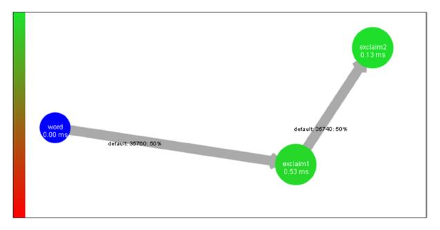
Figure 6-10. Storm user interface showing topology structure
