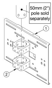
Slide the collars (Part 2) onto the pole, until the desired height is achieved.
