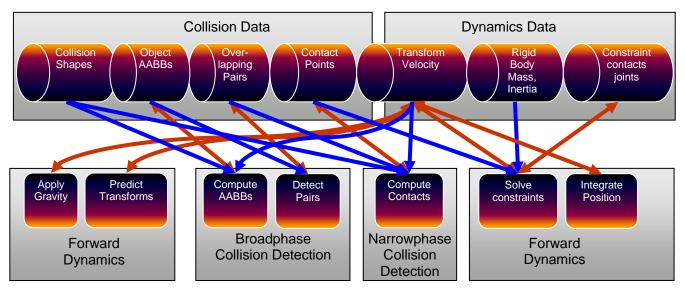
The entire physics pipeline computation and its data structures are represented in Bullet by a dynamics world. When performing 'stepSimulation' on the dynamics world, all the above stages are executed. The default dynamics world implementation is the *btDiscreteDynamicsWorld*.
