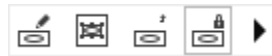
The PowerClip toolbar lets you edit, select, extract, lock, or reposition the contents inside the frame. The toolbar appears whenever a PowerClip object is selected.
