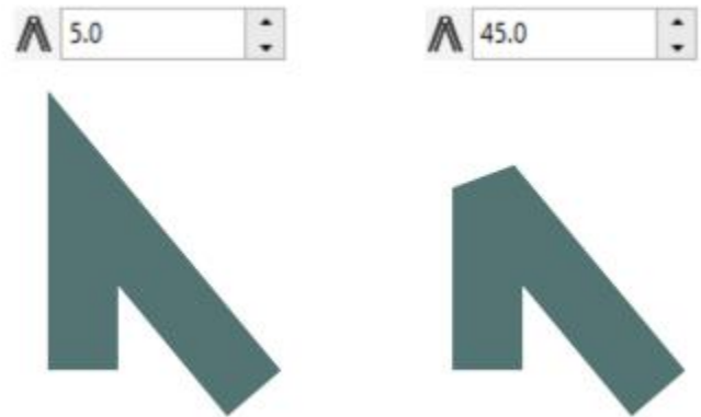
Lines meet at the same sharp angle. Left: The angle exceeds the miter limit, creating a pointed corner. Right: The angle is below the miter limit, creating a beveled corner.
