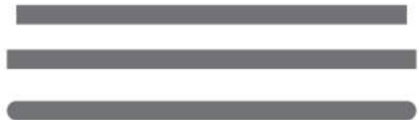
Line caps from left to right: Square cap, Extended square cap, and Round cap.
