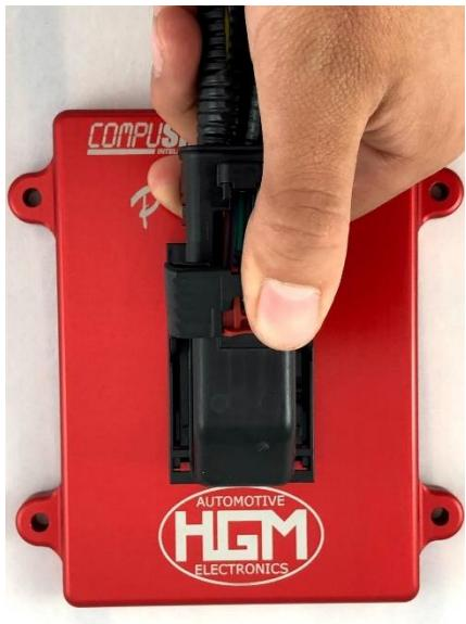
To remove the connector, pull the red tab up, then press down on the release panel.
