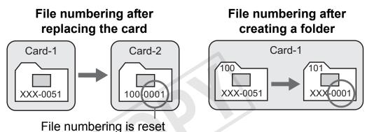
[Manual reset]: To reset the file numbering to 0001 manually or to start from file number 0001 in a new folder.
