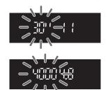
If the picture will be too dark, the "30"" (30 sec.) shutter speed display will blink. If this happens, turn the < > dial to the left to set a lower aperture f/number or increase the ISO speed.
