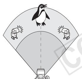
All the slave units will fire at the same output and be controlled to obtain a standard exposure.
