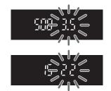
If the exposure will be too dark, the maximum aperture (smallest number) will blink. If this happens, turn the < > dial to the left to set a slower shutter speed or increase the ISO speed.
