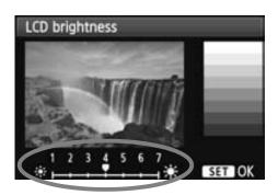
Under the [**Y**<sup>2</sup>] tab, select [**LCD brightness**], then press < (SET) >. With the adjustment screen displayed, press the < ►> key to adjust the brightness, then press < (SET) >.
