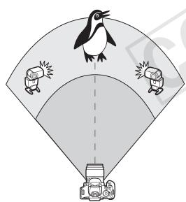
Convenient when you need a large flash output. All the slave Speedlites will fire at the same output and be controlled to obtain a standard exposure.
