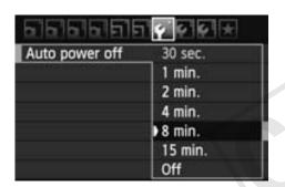
Under the [¶¹] tab, select [Auto power off], then press < (SET) >. Select the desired setting, then press < (SET) >.
