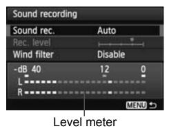
Normally, the built-in microphone will record monaural sound. Stereo sound recording is possible by connecting an external microphone equipped with a stereo mini plug (3.5mm dia.) to the camera's external microphone IN terminal (p.18). When an external microphone is connected, sound recording will switch automatically to the external microphone.
