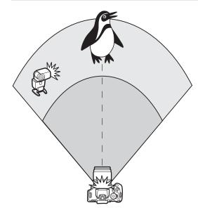
This describes fully-automatic wireless flash shooting with one external Speedlite and the built-in flash.
