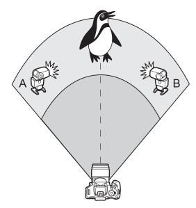
Divide the slave units into groups A and B, and change the flash ratio to obtain the desired lighting effect.
