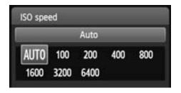
If the ISO speed is set to [AUTO], the actual ISO speed to be set will be displayed when you press the shutter button halfway. As indicated below, the ISO speed will be set automatically to suit the shooting mode.
