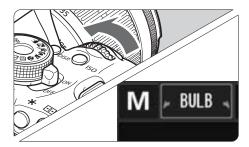
A bulb exposure keeps the shutter open for as long as you hold down the shutter button. It can be used to photograph fireworks, etc.
