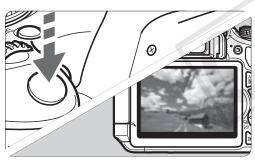
Press the shutter button completely to take the picture.
