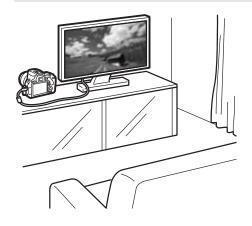
Use the provided AV cable or an HDMI Cable HTC-100 (sold separately) to connect the camera to a TV set. Then you can playback the captured movies and still photos on the TV. If you have a High-Definition TV set and connect your camera with an HDMI cable, you can watch Full High-Definition (Full HD: 1920x1080) and High-Definition (HD: 1280x720) movies with higher image quality.
