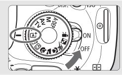
Set the power switch to <ON>, and set the Mode Dial to  $<\triangle^{\dagger}>$  (Scene Intelligent Auto). (p.50)
