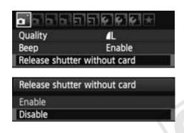
If there is no card installed and you press the shutter button, "Card" will be displayed in the viewfinder, and you cannot release the shutter.
