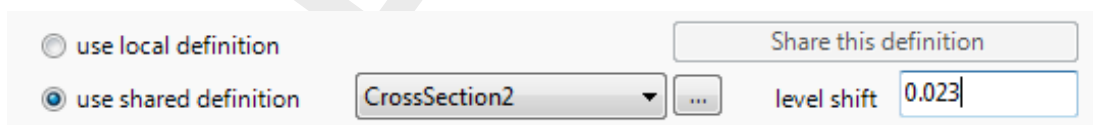
Figure 4.32: Switch between Local Cross Section definition and Shared Cross Section definition in the Cross Section editing window
