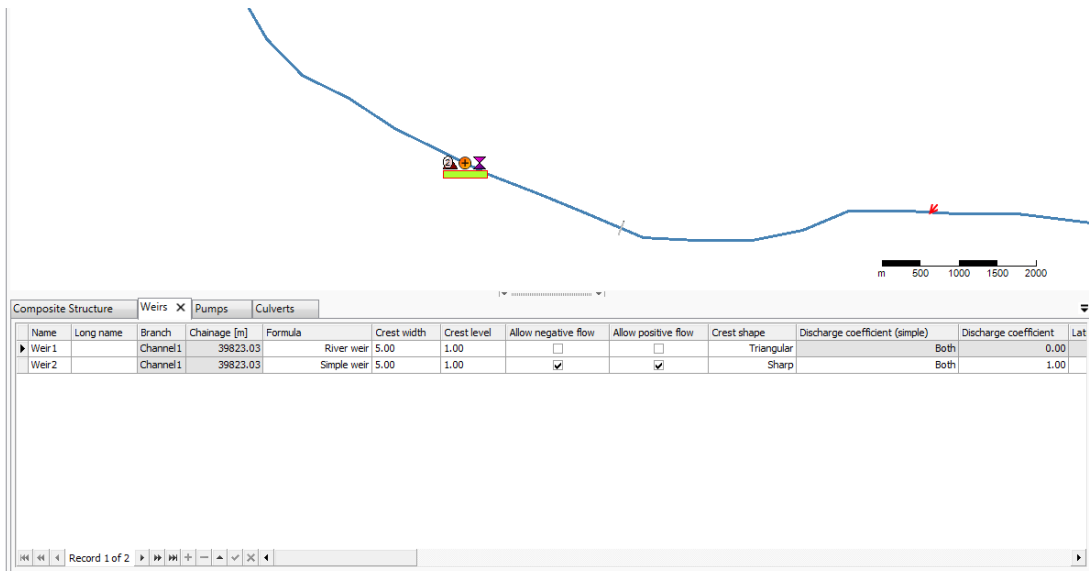
Figure 4.22: Example of a Composite Structure in the Central Map. Multiple structure objects (here: two Weirs, a Pump and a Culvert) are arranged horizontally, the bar below the structure icons indicates that the structures are combined to a Composite Structure. The Attribute Table lists the sub-structures of Weir type
