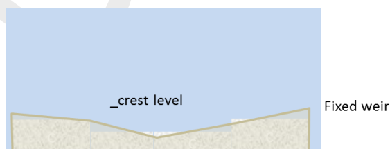
Figure 4.16: Schematic representation of a fixed weir
