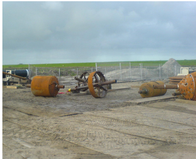
Figure 1.4: Reamer and cutting wheel
