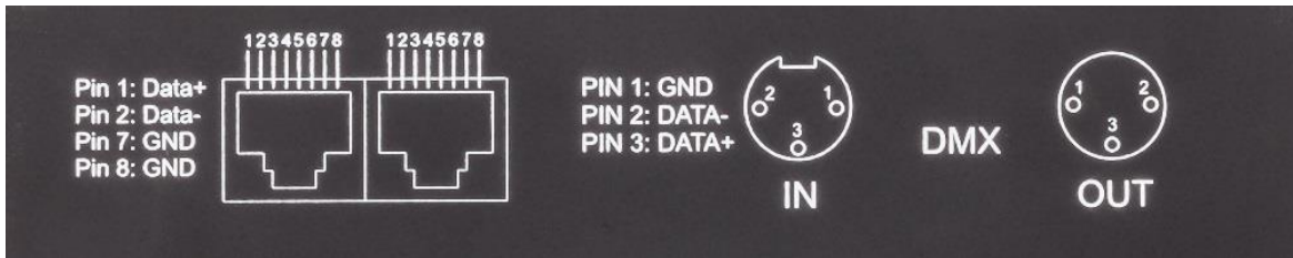
Figure III: Connector Pinout for DMX-4-5000-3-10A
