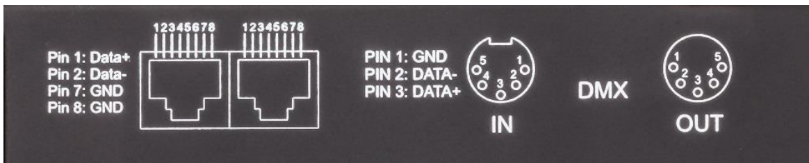
Figure IV: Connector Pinout for DMX-4-5000-5-10A
