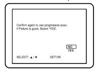
Confirm your setting, then press OK. The menu will disappear and PROGRESSIVE will be ON. If you do not press any buttons for 15 seconds, Progressive Scan will switch to OFF.
