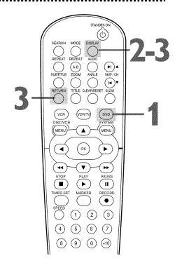
Press DISPLAY repeatedly or press RETURN to remove the display.
