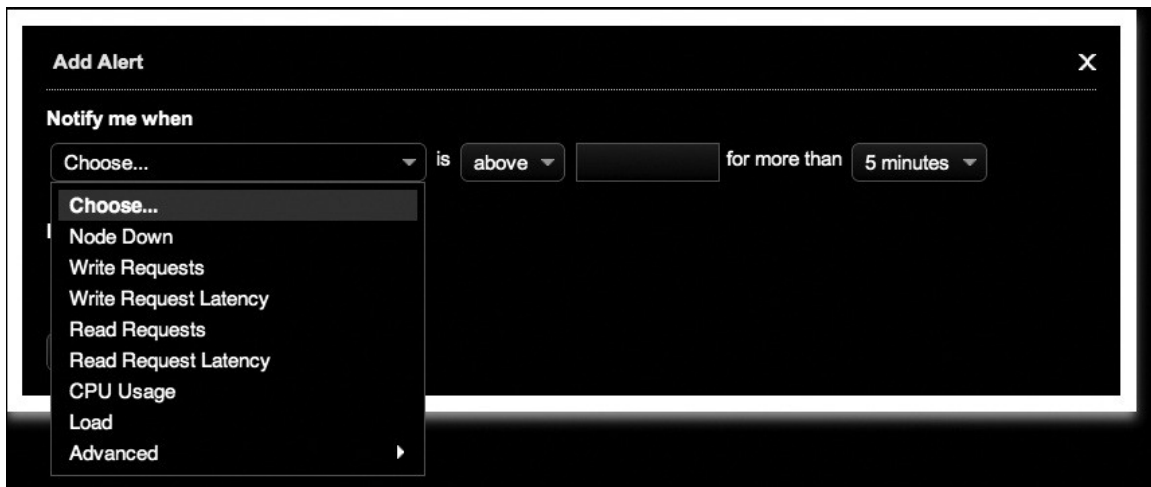
Figure 14 - Creating an alert in OpsCenter.
