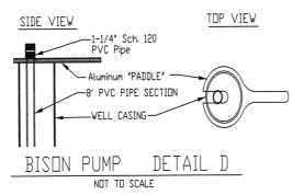
**STEP #10** - Lower the cylinder and the first 8' section of piping into the well. Using the slotted aluminum paddle you received with your pump, slide it under the PVC bell end of the pipe and rest the paddle on top of the well casing. This will hold the pipe in place while you assemble the rod and pipe. Continue to connect the 3/8" rod sections and PVC pipe until you have lowered all of the pipe into the well.
