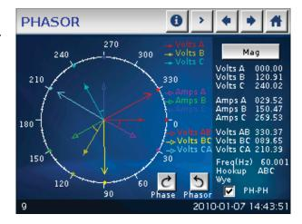
• The **PH-PH** check box shows/hides the phase to phase voltage.
