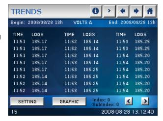
NOTE: If password protection is enabled for the meter a keyboard screen displays, when you press any channel button. Use the keyboard to enter the password. If a valid password is entered, the Trend graphic/ Tables are displayed; otherwise a message displays, indicating that the password is invalid.
