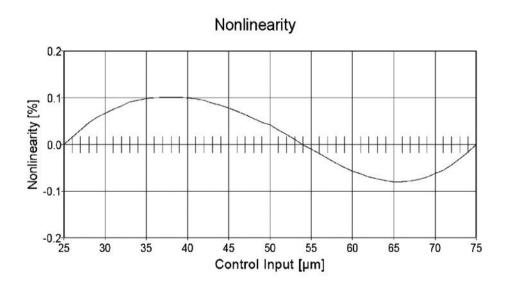
Excellent linearity thanks to the combination of E-852 evaluation electronics and D-510.050 sensor (in the nominal measuring range)
