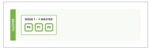
Figure 2-2. A single-node cluster with an index
