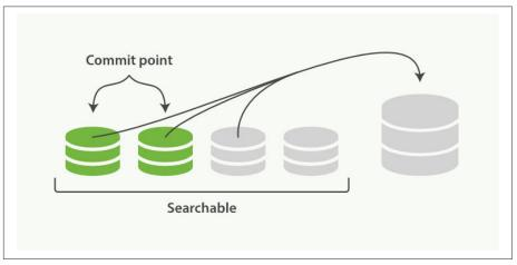
Figure 11-10. Two committed segments and one uncommitted segment in the process of being merged into a bigger segment
