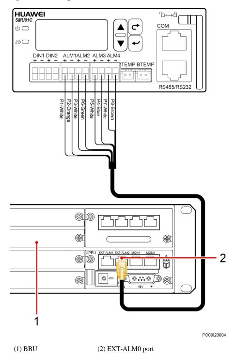
Figure 4-9 Connecting the SMU01C and the BBU
