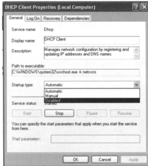
Figure 1.6 You Can Disable a Windows Service by Right-Clicking the Service in the Windows Services Console and Selecting Properties
