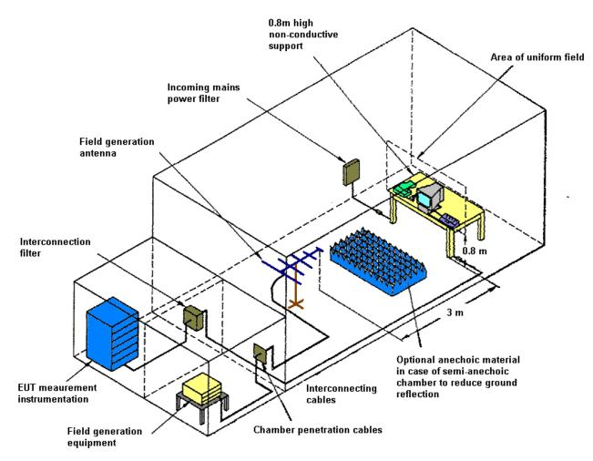
NOTE: The chamber is compliance with the sixteen points uniform field requirement as stated in IEC 61000-4-3 Section 6.2.
