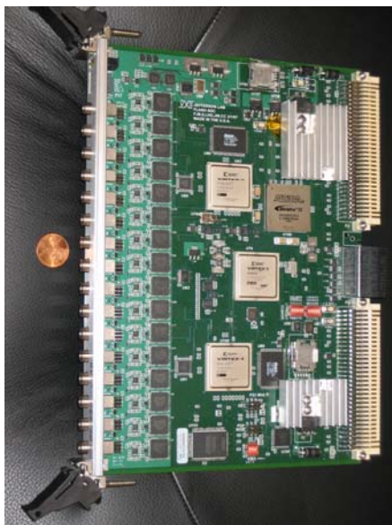
Figure 3: The 250 MSPS fADC
