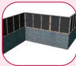
fig 7 Showing moisture barrier and battens before the cladding begins
