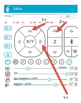
• Start with SMALL increments first to verify movement in the correct direction. X+ moves the print carriage to the right, Y+ moves the bed forward toward the front, Z+ moves the print carriage up. If any of the axes go in the wrong direction, turn the connector on the board 180 degrees for that axis.
