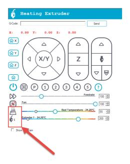
After a few seconds, you should notice the temperatures on both the hot end and heated bed starting to rise. Also, the fan on the power supply may start up. That's normal. There will also be red LED indicators on the controller board.
