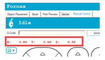
• If the values are not zero <u>and you have homed the hot end</u>, you will have to zero them out manually. The best way to ensure these values are zeroed out is to remove both the power and the USB cable from the controller. On the CLUB you remove power by disconnecting the power supply from the wall outlet.
