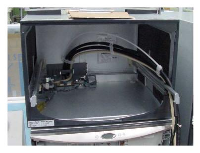
It is also a good idea to push the hoses and the link support down while re-fitting the wiring cover. This ensures that the link support does not interfere with the tub when the drawer is closing. If the hoses have become twisted in the link support, or if the link support is too close to the tub, this can cause drawer closing problems. Either the drawer will not close fully or will close slowly over the last 35 mm. (1 ½ inches)
