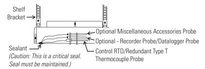
Figure 1-3. Chamber Probe(s)
