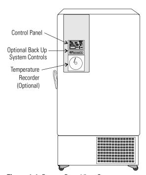
Figure 1-1. Freezer Front View Components
