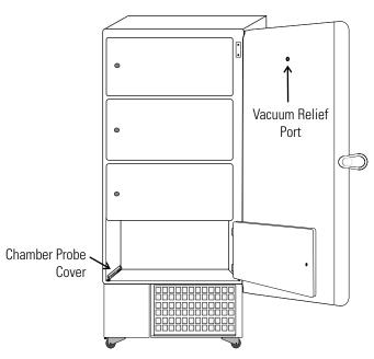
Figure 1-4. Vacuum Relief and Probe Cover Location
