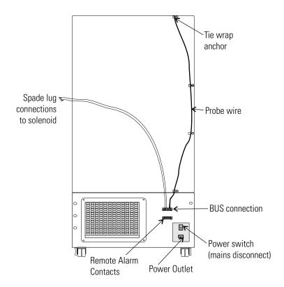
Figure 5-5. Probe wire and solenoid connections
