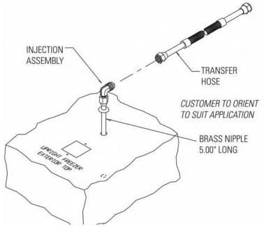
Figure 5-1. Injection Assembly
