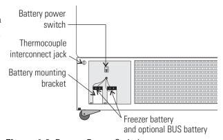
Figure 4-2. Battery Power Switch
