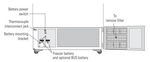
Figure 1-5. Battery(s) location and switch
