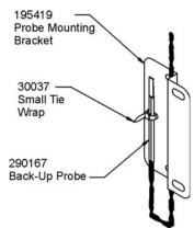
Figure 5-3. Secure probe
