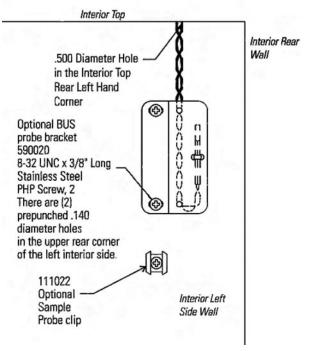
Figure 5-4. Mounted probe clip
