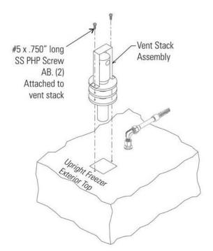
Figure 5-2. Vent Stack Assembly
