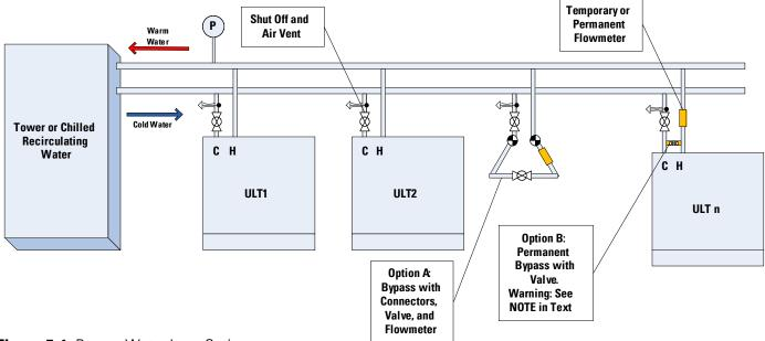
Figure 5-1. Bypass Water Loop Options
