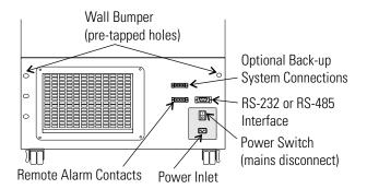
Figure 1-2. Freezer Rear View Components
