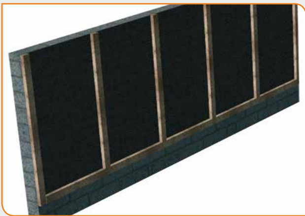
fig 1 Showing moisture barrier and battens before the cladding begins
