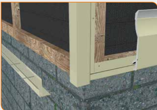
fig 2 Showing starter trim and showing the use of the universal corner trim for external angles
