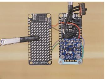
Use two **M2x8mm** screws so they can reach through the Feather and in the 3d printed spacer.
