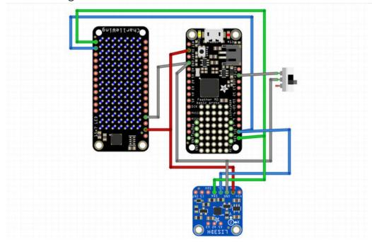
Take a moment to review the components in the circuit diagram. This illustration is meant for referencing wired connections - The length of wire, position and size of components are not exact.
