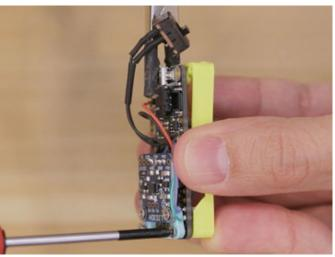
First fasten the two screws on the accelerometer mount. Leave the other two screws unfastened until we fit the battery cable through the opening on the spacer.
