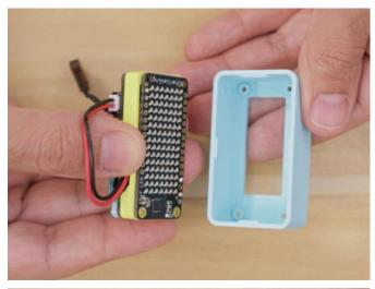
One side of the enclosure is wider to accommodate the JST connection on the side of the Feather board. Carefully fit the wires inside the enclosure. You can use tweezers to arrange them next to the spacer.
