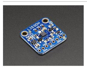
Adafruit LIS3DH Triple-Axis Accelerometer (+-2g/4g/8g/16g)
