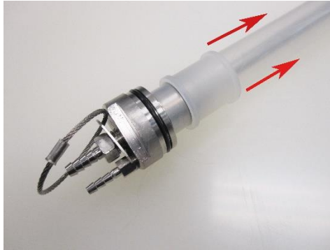
Figure 4-3: Removal of upper HDPE Compression Ring
