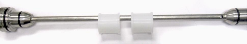
Figure 4-13: Compression rings on the center tube weldment
