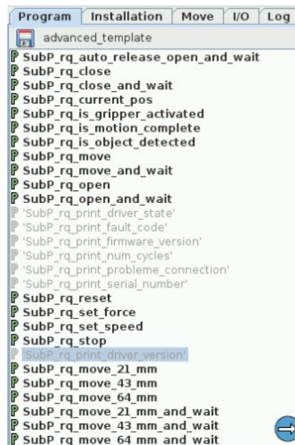
Fig. 4-15: Older program's subprograms to suppress or rename to use with URcaps package.
