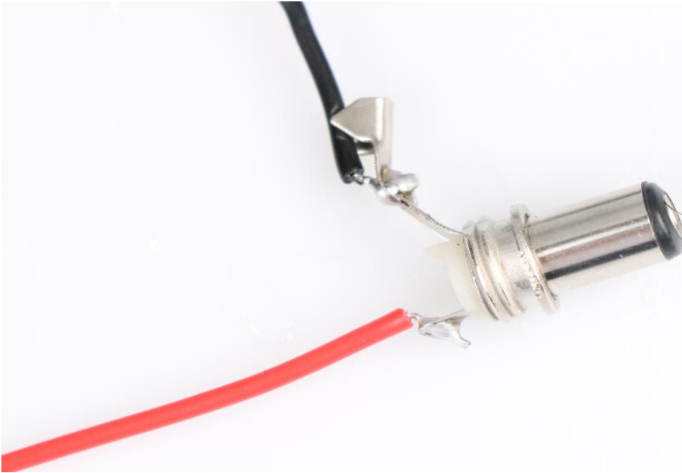
Fig.3.1.32. Wire welding schematic
