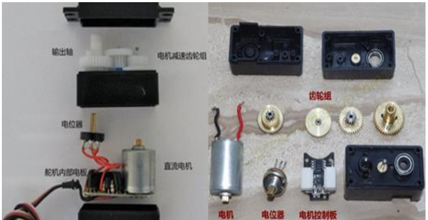
Fig.3.2.23 Composition of Steering Gear
