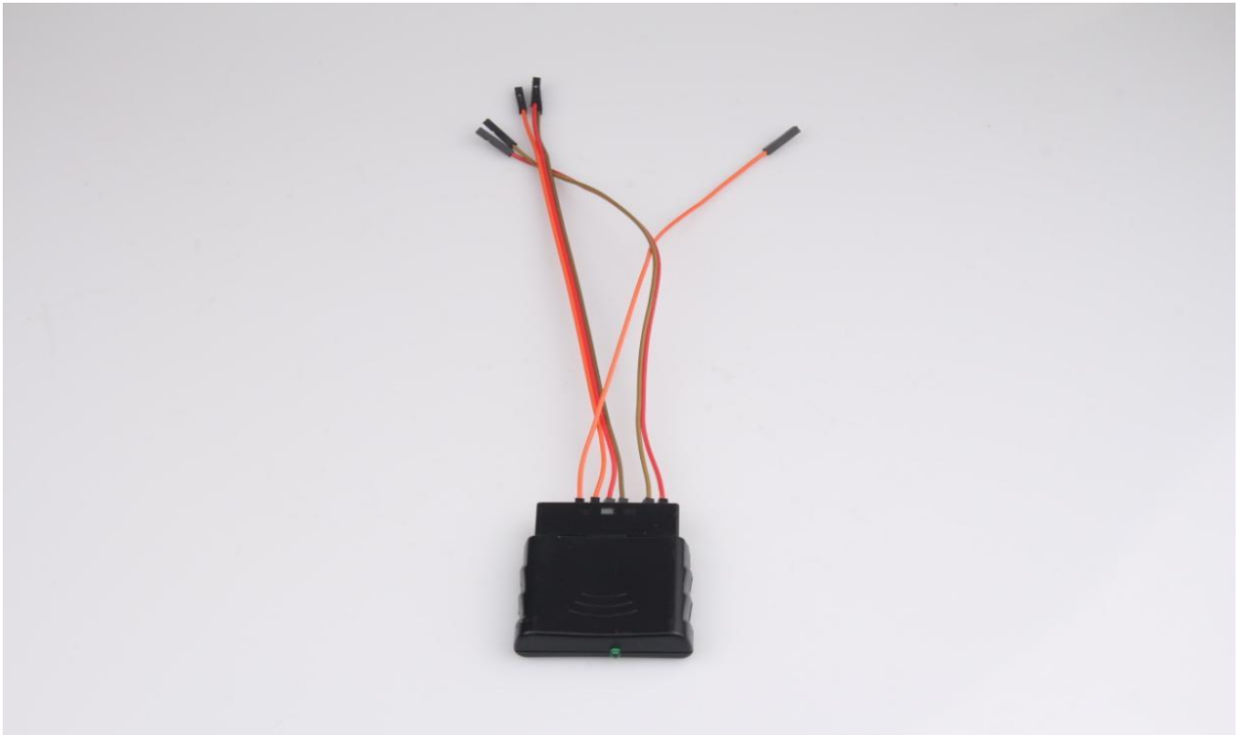
Fig.3.2.41 Wiring of the Receiver Head
