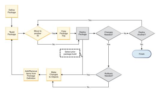
Figure 2. Deployment package workflow
