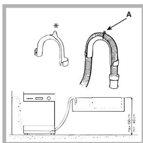
The special plastic elbow\* makes it easier to find the best layout: fix the elbow to the wall securely in order to prevent the outlet hose from moving and spilling the dirty water. The part of the hose marked with the letter A should be between 40 and 100 cm above the ground (see figure).
