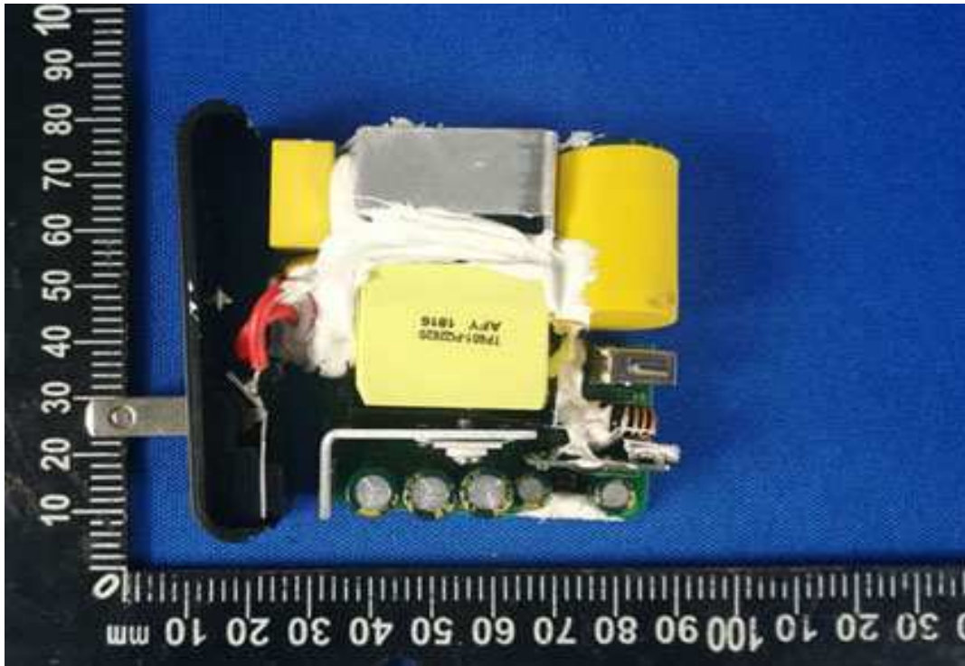
Photo 19 - PCB components view: TP452CA, TP601CA, TP451CA, TP301CA and TP302CA
