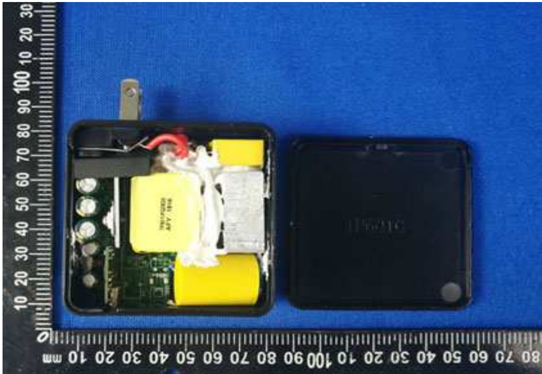
Photo 21 - Internal view of the unit TP601C, TP451C, TP301C
