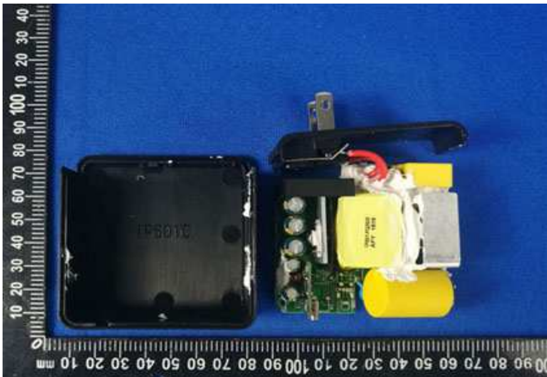
Photo 22 - Internal view of the unit TP601C, TP451C, TP301C
