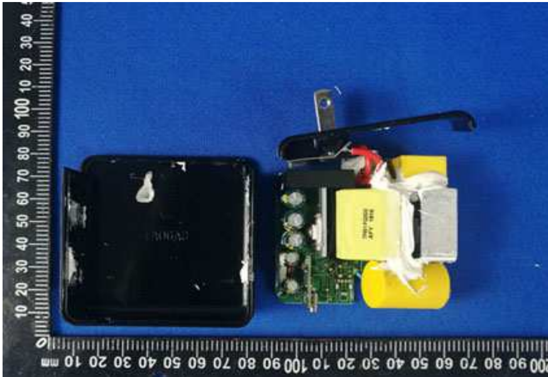
Photo 27 - Internal view of the unit TA06A3 and TA07E3
