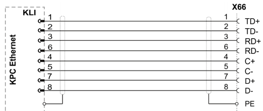
Fig. 6-11: Connector pin allocation X66
