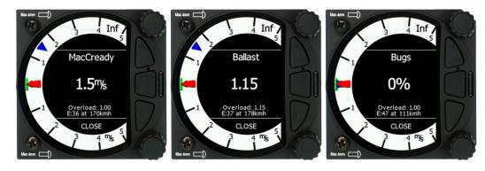
Rotate the bottom knob to modify any setting. Next check the safety altitude (height above destination, arrival altitude) setting.
