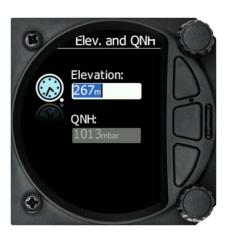
The instrument will offer elevation over standard pressure level QNE. Use the knob to finetune the elevation.
