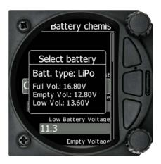
Alternatively, you can manually change the Full Voltage, Low Battery Voltage and Empty Voltage if your battery type is not listed. Those settings will influence the battery level icon and low battery warning.
