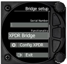
NMEA output is used to transmit NMEA sentences. You can select desired NMEA sentences and define baud rate at which they will be transmitted.
