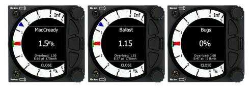
To change the McCready value press the bottom rotary knob and press on MC/BAL. A short press of the lower rotary knob moves from McCready to the Ballast box and pressing the lower rotary knob again will open the Bugs box. If no action is performed within 3 seconds, the box will close, or you can also press CLOSE anytime (lower push button).
