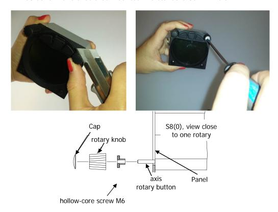
Remove the two rotary knob caps with a knife or flat screw driver, then hold each knob and unscrew it. Remove the remaining two screws and the two M6 threaded nuts. Install the S8x/S10x into the panel and screw back all screws, nuts and knobs. Ensure that between the knobs and the panel there is sufficient space so that the button can be pushed.
