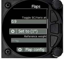
When all flap positions are set, a green dot will be displayed with current flap position. If flap labels are not set yet, press **EDIT** to name label. Flap labels must be entered with increasing speed range. It is recommended that flaps labels are set together with speed range in Polar and Glider setup. It is also possible to toggle between cruise and climb mode using the flap sensor.
