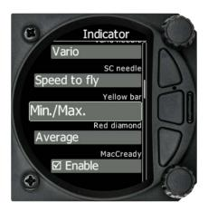
**Vario Needle:** Can be set to Vario, SC, Netto or Relative. **SC needle:** Can be set to Vario, SC, Netto or Relative.
