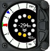
The central number and chevrons indicate if the Flarm target is below or above and by how many meters/feet. The number in the bottom right indicates the range in meters/feet. The numbers are related only to the closest or the most dangerous target.
