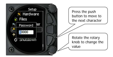
Once the required value is selected, press the lower push button to move to the next character selection. To move back to the previous character, press the upper push button. When you have finished editing, press the Enter key – the lower rotary button. A short press of the middle push button exits from the edited field ("control").
