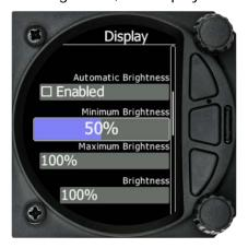
With a push of the lower rotary button you can activate the slide control and then by rotating the knob you can select the preferred value and confirm it via the push button.
