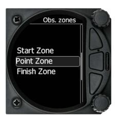
The Start, Waypoint and Finish zone can be configured separately although the setup is very similar.
