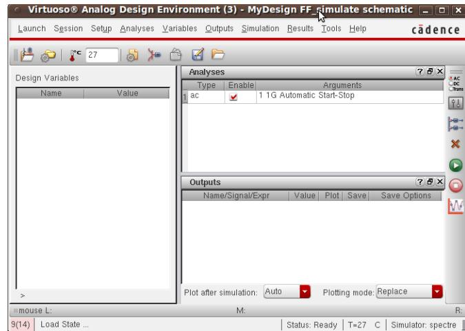
To calculate input sink capacitance, we need to get current waveform which depicts current following into the input D. In your schematic, the sinusoidal voltage source (**vsin**) is attached to the input D, therefore we need to see the current from **vsin**.
