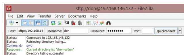
Figure 95: Using Filezilla to connect from a Windows computer to a Linux FTP server with SFTP
