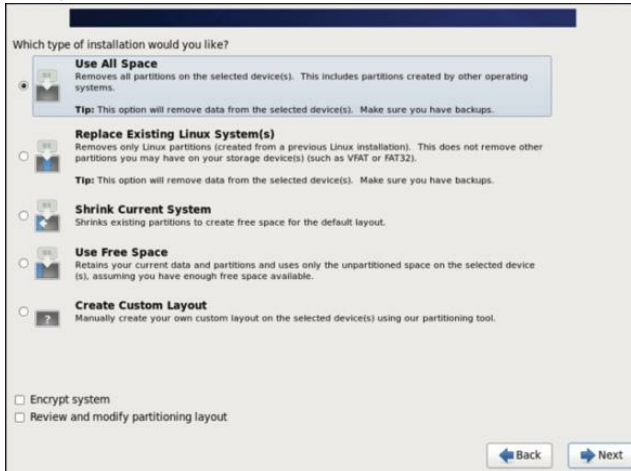
Figure 13: Choosing the type of installation for the disk(s)
