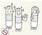
Use only specified standard batteries. Do not use new and used batteries together.
