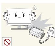
Remove the vinyl cover of the adapter before using the adaptor.
