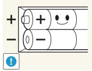
When replacing the batteries, insert them with right polarity (+, -).
