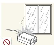
Do not let water enter the DC power device or get the device wet.
