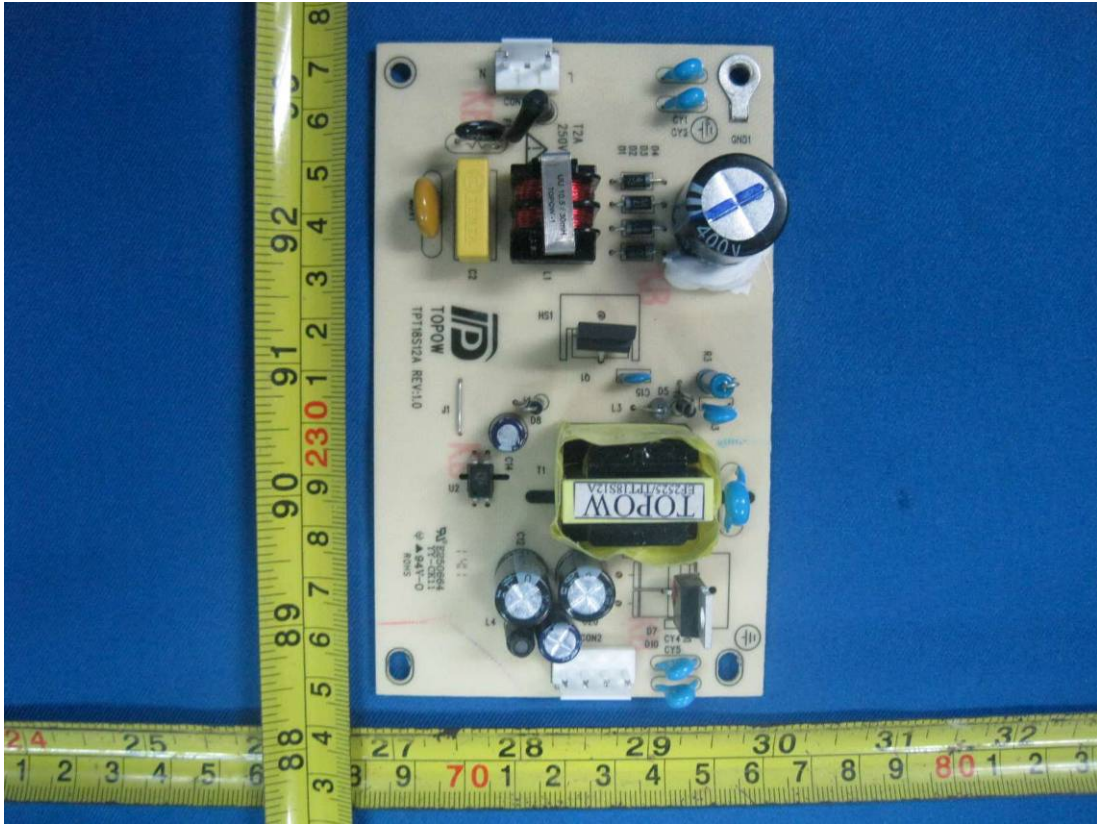
Fig. 9 – Top view of power board (model: TPT18S12A)
