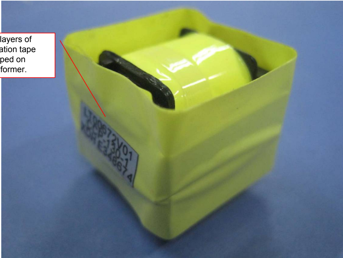
Fig. 13 – Transformer T1 on power board (model: G0682) overview(1)
