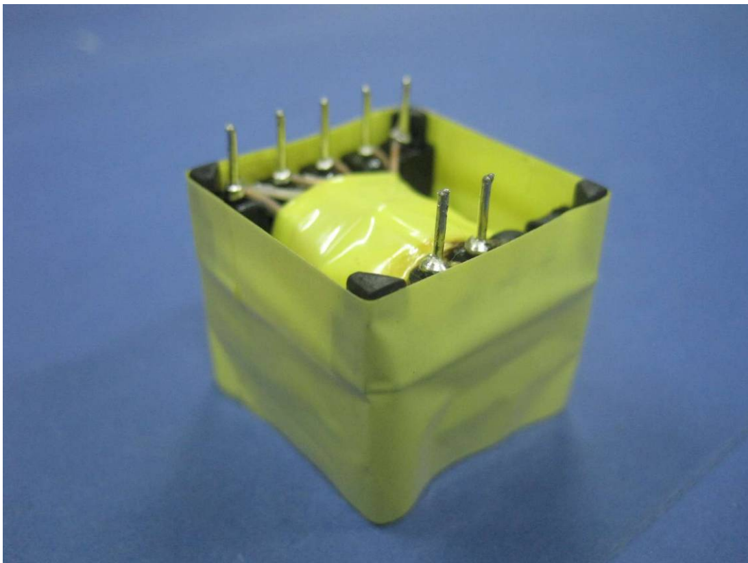
Fig. 14 – Transformer T1 on power board (model: G0682) overview (2)
