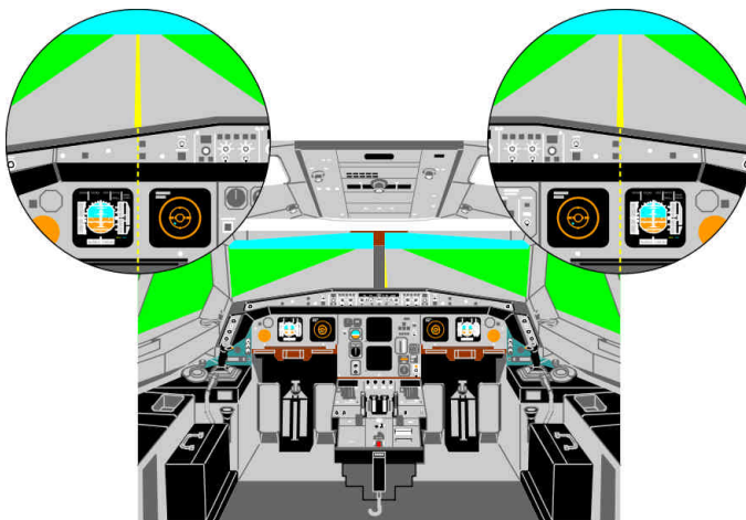
Proper Centerline Following
