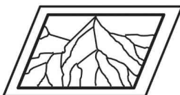
Outer Ply Cracking
