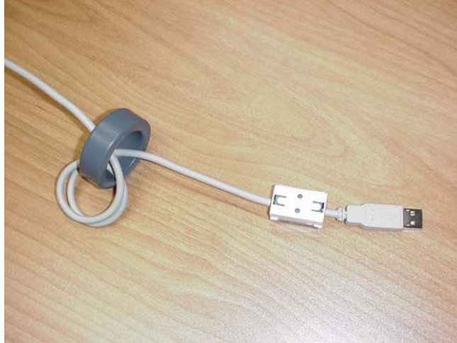
Figure 8 - Example of a USB Cable Using Ferrites
