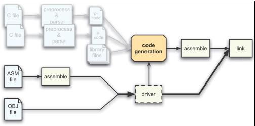
FIGURE 4-4: COMPILATION SEQUENCE WITH ASSEMBLY FILES
