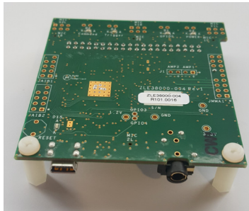
Figure 4 • ZLE38AVS board with standoffs attached
