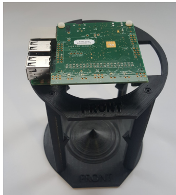
Figure 5 • ZLE38AVS board attached to mounted Raspberry Pi
