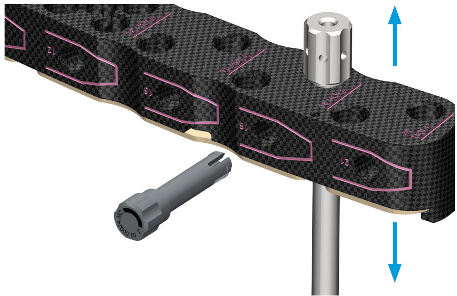
Fig. 7 Adjust the height of the Targeting Device to allow Safety Lock Pin placement.
