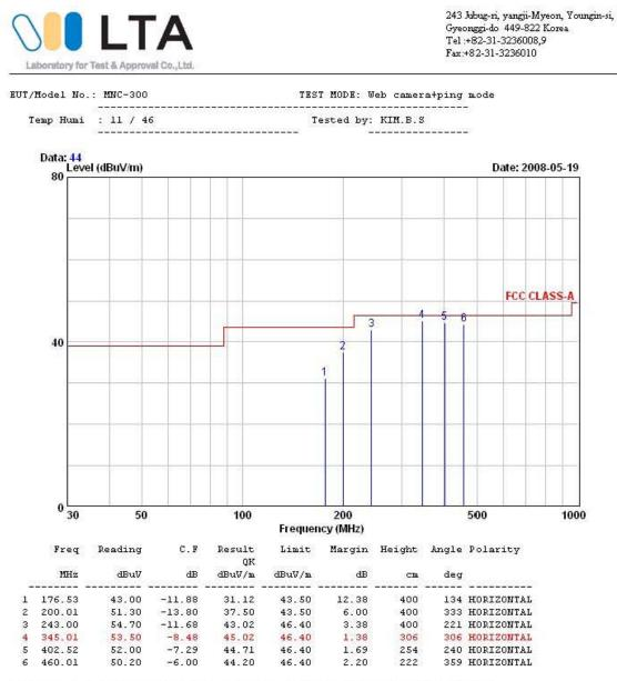
Remarks: C.F (Correction Factor) = Antenna factor + Cable loss - Preamp gain
