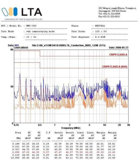
Remarks: C.F (Correction Factor) = Insertion loss + Cable loss
