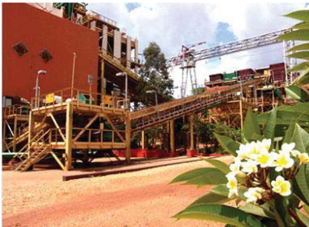
Mining conveyor at the Catoca Diamond Plant - The fourth largest diamond mining plant in the world. Motor size: 140A at 6600V
