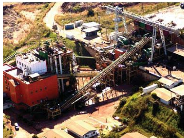
Mining conveyor at the Catoca Diamond Plant - The fourth largest diamond mining plant in the world. Motor size: 140A at 6600V
