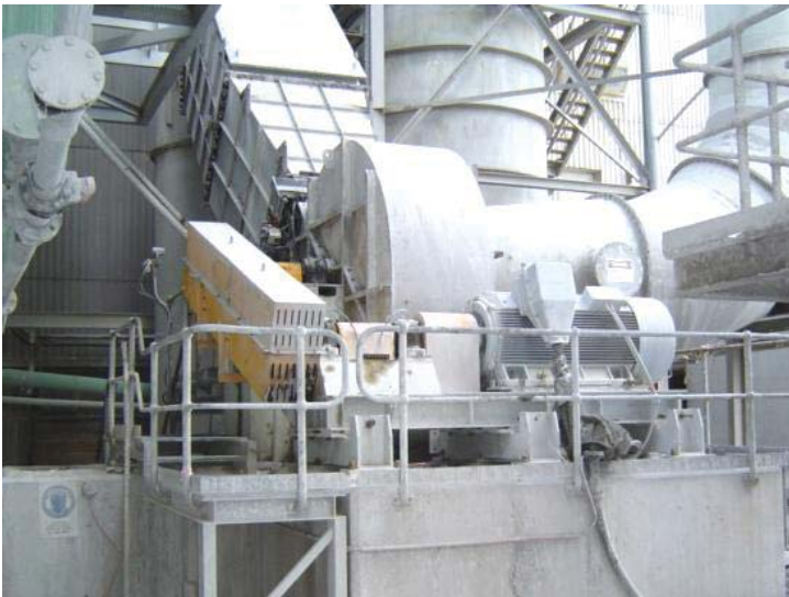
Scrubber blower in the Incitec Pivot fertilizer plant in Queensland, Australia. Motor size: 250A at 6600V
