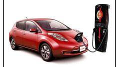
The earlier options take hours for a car to recharge. Fast chargers by comparison take much less time, and make long distance road trips practical. They work by providing a much greater amount of electricity and by changing it into *direct current* meaning it can be fed straight into the battery. Like petrol, you can choose just to 'top up' your car and put in a few minutes' worth of power.
