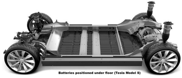
Battery size is measured in kilowatt-hours, or kWh. Lower priced electric cars have ~24 kWh batteries; high-end Tesla cars have up to 100 kWh; buses and trucks much more still. This affects range and cost.
