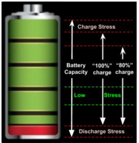
The life of a battery is reduced when at extreme high or low levels of charge<sup>40</sup>. To avoid cars reaching either end, not all of the battery capacity is made available.
