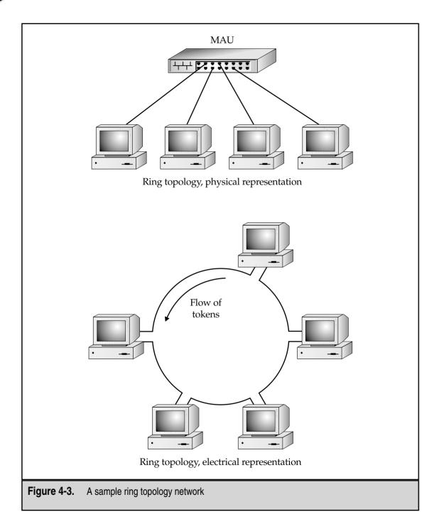
Ring topology LANs are based on Token Ring instead of Ethernet. Some may also run Fiber Distributed Data Interface (FDDI)—a 100Mbps fiber-optic network. Rings are also used for some larger telecommunications networks such as Synchronous Optical Network (SONET).
