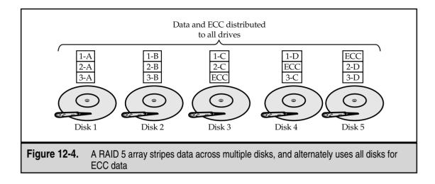
Which level of RAID should you use on your network server? Most network administrators favor RAID 5 because it requires only 20 to 25 percent of the total disk capacity for the redundancy function. Yet it performs well and offers a measure of safety. However, RAID 3 and RAID 5 arrays do occasionally fail to recover data properly (although they very rarely lose data). For this reason, you usually should opt for either RAID 1 or RAID 10 for network servers that store important data.
