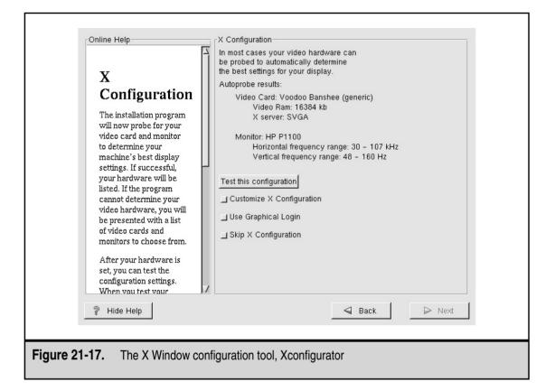
Four choices exist under the description of the hardware configuration: Test the configuration, customize the X configuration, use a graphical login, and skip the X configuration.
