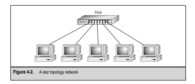
of the nodes connected to the hub is using half the available bandwidth, all the other nodes must contend with that use for their own. In other words, if you're using a network type with a capacity of 10Mbps, that's the total amount of bandwidth available to all nodes connected to the hub in aggregate.
