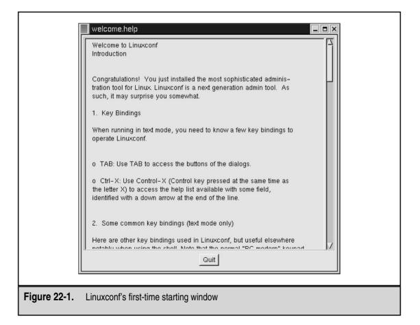
When you're done reading the window's text, simply click the Quit button at the bottom of the window to exit the introduction screen and start Linuxconf for reading. The opening window to Linuxconf will look like Figure 22-2.
