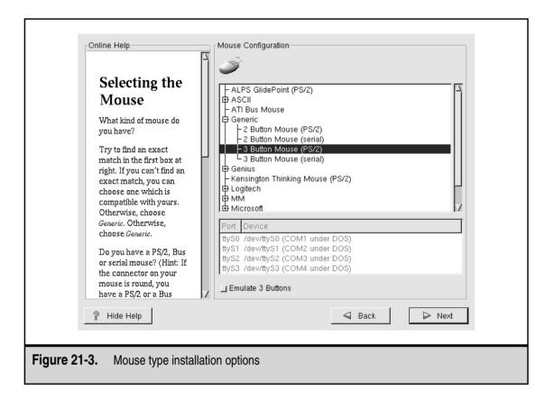
If you have a two-button mouse, you want to click the Emulate 3 Buttons checkbox at the bottom of the screen. This is because some features of the X Window environment work only with a three-button mouse. By selecting this checkbox, you can click both buttons of a two-button mouse to emulate the middle button.
