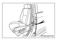
For the GAWR, see the Certification Label. For the maximum load of the tire, see the load limit at maximum cold tire inflation pressure mentioned on the sidewall of the tire. (→P. 528)
