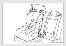
Seat belts equipped with a child restraint locking mechanism (ALR/ELR belts except driver's seat belt) ( $\rightarrow$ P. 69)
